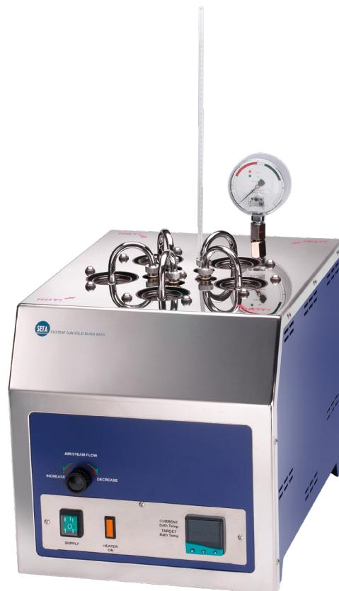
A Solid Block Bath designed to carry out up to five simultaneous tests for determining existence gum content in fuels by the Jet Evaporation method.
